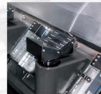
Parts Supporting Device Offer stable support to the long workpiece.
