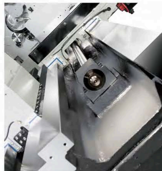
The major machine parts, such as the base, saddle, headstock, slide and tailstock are made of Meehanite cast iron and tempered to relieve stress thereby ensuring lifetime accuracy.
